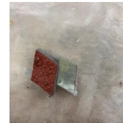
Piece on the left shows adhesion qualities of permanent foaming fixative to substrate, 2nd piece shows no adhesion qualities to substrate
