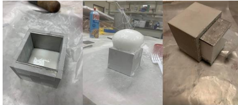
Adhesion Samples Fabrication
