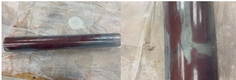
Left picture: Encapsulation pipe experiment conducted at FIU-ARC; Right picture: Simulated contamination (green) inside pipe with foam (red)
