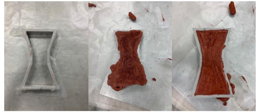
Rigid Foam Fabrication Process
