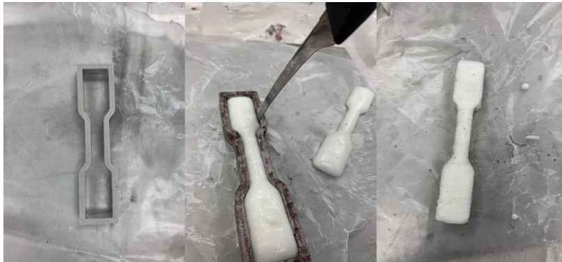
Flexible Foam Fabrication Process
